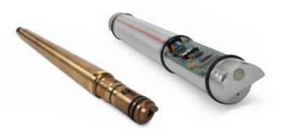
Gamma ray tools record naturally occurring gamma rays in the formations adjacent to the wellbore. This nuclear measurement indicates the radioactive content of the formations. Effective in any environment, gamma ray tools are the standard device used for the correlation of logs in cased and open holes.
